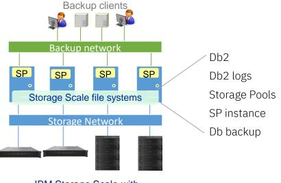
IBM Storage Scale with ESS3000 and ESS3500
