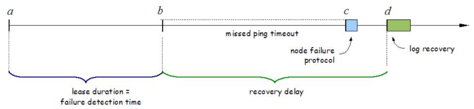
The length of a non-quorum node's lease (in seconds) is defined by the configuration options **leaseDuration** and **failureDetectionTime**. Based on IBM test experience, we recommend always tuning **failureDetectionTime** and never **leaseDuration** (setting **failureDetectionTime** will also change **leaseDuration**).
