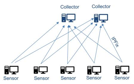
Setting "Collector Redundancy" to 2 will ensure that the performance data is mirrored to two collectors
