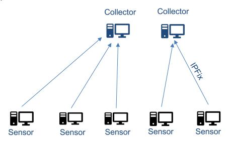
Sensors gather the performance metrics from Spectrum Scale components, Linux, etc. and send it through the IPFix protocol to collectors
