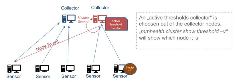
Node specific threshold events are forwarded to the corresponding node and shown there in mmhealth. Cluster wide threshold events will be shown on the active threshold monitor node.
