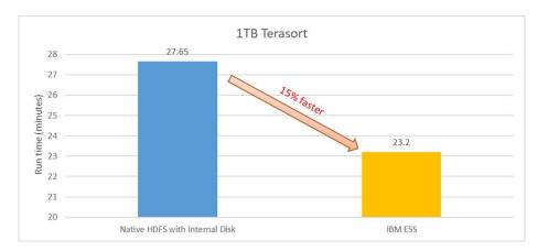
ESS based shared storage setup performed 15% faster compared with native HDFS with internal disks.
